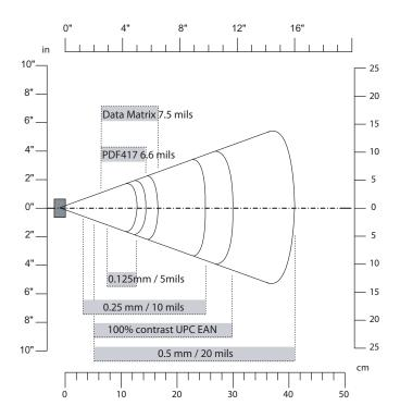
**2D Area Imager Minimum Reading Distances:** This graphic does not include the 0.180 cm (0.071 in) setback for the SR61.
