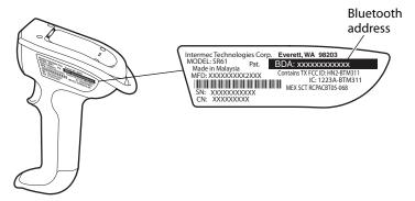
**SR61 Bluetooth Address:** The SR61 Bluetooth address is located in the top right corner of the label on the side of the SR61.
