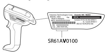
**SR61 Scan Engine Option:** The scan engine option of your SR61 is the sixth character of the configuration number. In this illustration, the scan engine option is V or 1D linear imager.
