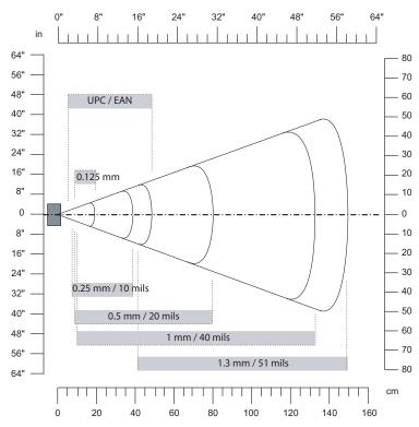
**Standard Range Laser Scanner Minimum Reading Distances:** This graphic does not include the 0.260 cm (0.102 in) setback for the SR61.
