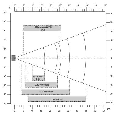
**Linear Imager Minimum Reading Distances:** This graphic does not include the 0.255 cm (0.100 in) setback for the SR61.
