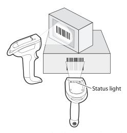
**Scanning Bar Codes:** The aiming and scanner beams that you see depend on whether you have a laser scanner (SR61xL), 1D linear imager (SR61xV), 2D area imager (SR61xA), or near-far range area imager (SR61xE).
