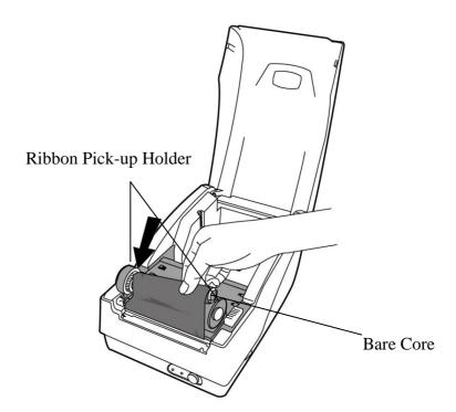
8. Turn the wheel of the print head module to ensure the ribbon is tightly wound.
