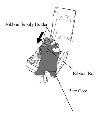
7. Turn back the print head module and then insert the bare core into the pick-up holder. (First snap in the left side, and then the right side.)
